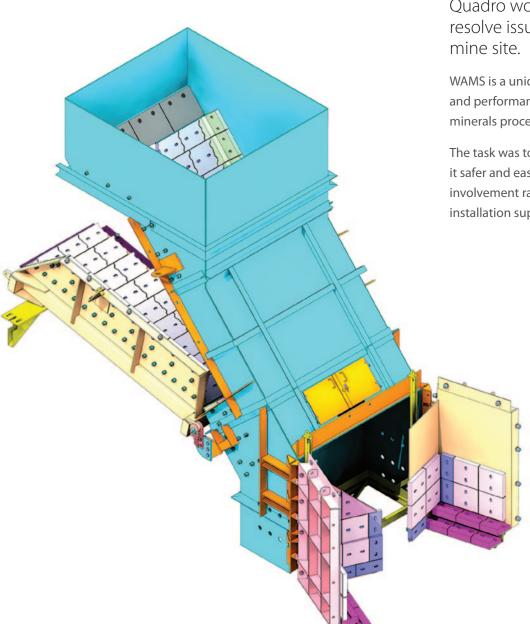
Quadro worked in conjunction with WAMS Pty Ltd to resolve issues with a Tripper chute at the Paraburdoo mine site.
